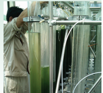
ENN mobile algae photobioreactor testing platform.
